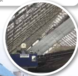
Berth E14 and E16 at the Bulk & General Cargo Terminal No.1 of Taipei Port has automated spiral coal and gravel unloader and conveyor system to mitigate dust concerns.
