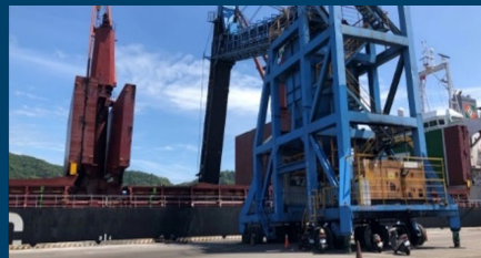
Automated coal unloaders and mist sprayers: enhance operational efficiency and reduce fugitive dust emissions
