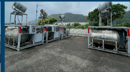
Automated coal unloaders and mist sprayers: enhance operational efficiency and reduce fugitive dust emissions
