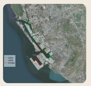
Schematic diagram of risk assessment of physical damage and functional loss of wharves and breakwaters exposed to strong winds due to vessel collisions
